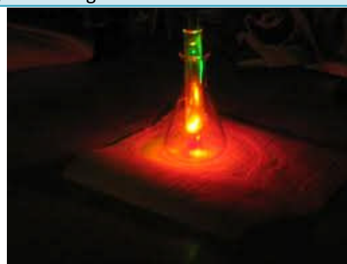
Alco Rhodamine B iluminated by green laser light 532nm
